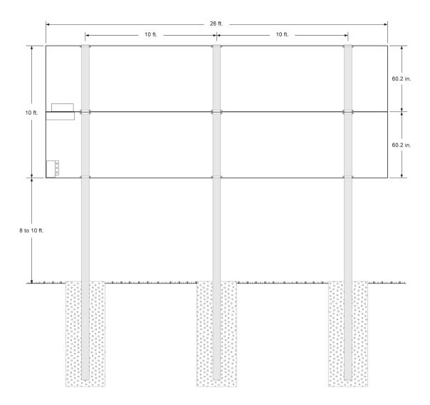
Once you have verified the positions of the posts and the size of the footings, you are ready to dig your holes, pour your concrete, and set your posts. There are several techniques for ensuring proper alignment of the posts. Typically installers will construct a temporary wooden support frame to hold each post in place while the concrete sets. Having plumb posts in the proper position is the key to a smooth mechanical installation.
